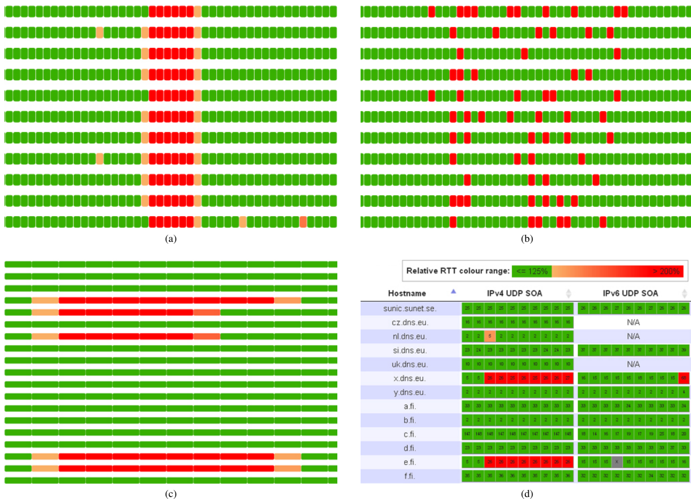
Figure 2. Examples of problem analysis. In (a), (b) and (c) the main matrix is represented, with x-axis (time) and y-axis (anchors) removed to obscure identities. (a) An outage where all anchors had severe problems reaching the server, causing a thick vertical band. (b) Partial denial-of-service attack, shown as a scattered vertical band. (c) Outage affecting a subset of anchors, with solid horizontal rows. (d) Recent measurements by an anchor.
